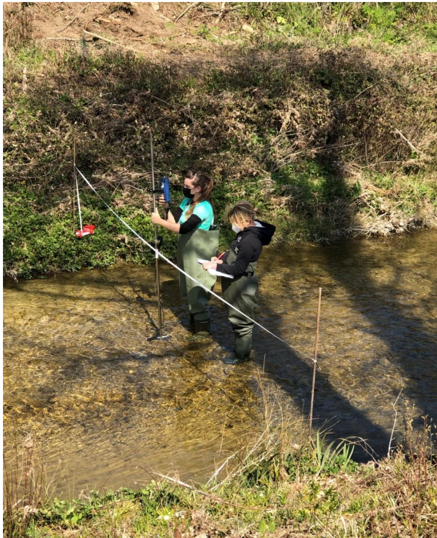
Figure 2. Measurement of the water flow rate on the Fossalto stream.
