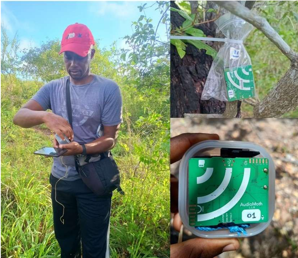
Photo 1: Principal Investigator (Martin Mwema) setting up audiomoth recorders
